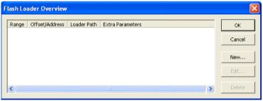
This dialog box lists all defined flash loaders. If you have selected a device on the **General Options>Target** page for which there is a flash loader, this flash loader is by default listed in the **Flash Loader Overview** dialog box.
