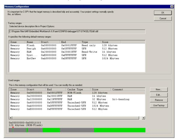
C-SPY uses a default memory configuration based on information retrieved from the device description file that you select, or if memory configuration is missing in the device description file, tries to provide a usable factory default. See *Selecting a device description file*, page 39.
