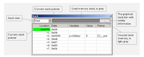
This window is a memory window that displays the contents of the stack. In addition, some integrity checks of the stack can be performed to detect and warn about problems with stack overflow. For example, the **Stack** window is useful for determining the optimal size of the stack.
