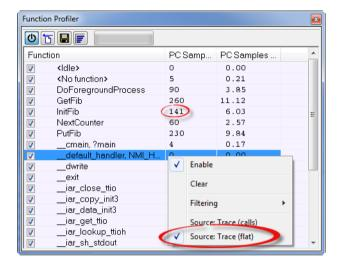
To secure valid data when using a debug probe, make sure to use the maximum trace buffer size and set a breakpoint in your code to stop the execution before the buffer is full.
