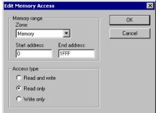
Use this dialog box to specify the memory ranges, and assign an access type to each memory range, for which you want to detect illegal accesses during the simulation.
