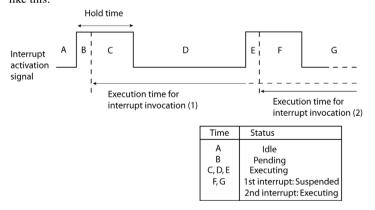
An execution time that is longer than the repeat interval might indicate that you should rewrite your interrupt handler and make it faster, or that you should specify a longer repeat interval for the interrupt simulation system.
