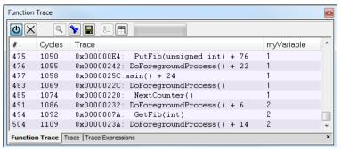
This window displays a subset of the trace data displayed in the **Trace** window. Instead of displaying all rows, the **Function Trace** window only shows trace data corresponding to calls to and returns from functions.
