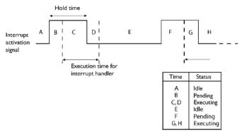
**Note:** The interrupt activation signal—also known as the pending bit—is automatically deactivated the moment the interrupt is acknowledged by the interrupt handler.
