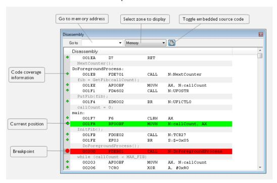
This window shows the application being debugged as disassembled application code.
