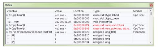
This window displays the values of variables with static storage duration that you have selected. Typically, that is variables with file scope but it can also be static variables in functions and classes. Note that volatile declared variables with static storage duration will not be displayed.
