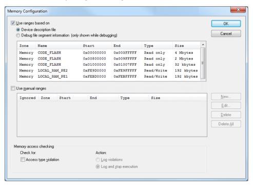
To handle memory as efficiently as possible during debugging, C-SPY needs information about the memory configuration. By default, C-SPY uses a default
