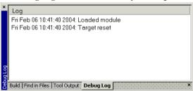
This window displays debugger output, such as diagnostic messages, macro-generated output, event log messages, and information about trace. This output is only available during a debug session. When opened, this window is, by default, grouped together with the other message windows, see *IDE Project Management and Building Guide*.
