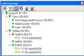
This window reports the status of the current code coverage analysis. For every program, module, and function, the analysis shows the percentage of code that has been executed since code coverage was turned on up to the point where the application has stopped. In addition, all statements that have not been executed are listed. The analysis will continue until turned off.
