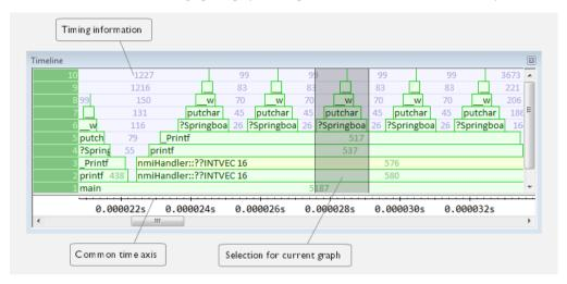
At the bottom of the graph you will usually find main, and above it, the functions called from main, and so on. The horizontal bars, which represent invocations of functions, use four different colors:
