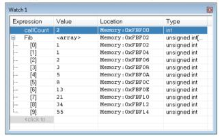
Use this window to monitor the values of C-SPY expressions or variables. You can open up to four instances of this window, where you can view, add, modify, and remove expressions. Tree structures of arrays, structs, and unions are expandable, which means that you can study each item of these.
