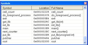
This window displays all symbols with a static location, that is, C/C++ functions, assembler labels, and variables with static storage duration, including symbols from the runtime library.
