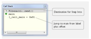
This window displays the C function call stack with the current function at the top. To inspect a function call, double-click it. C-SPY now focuses on that call frame instead.
