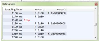
Use this window to view the result of the data sampling for the variables you have selected in the **Data Sample Setup** window.
