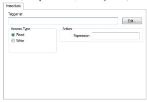
In the C-SPY simulator, use the **Immediate** breakpoints dialog box to set an immediate breakpoint. Immediate breakpoints do not stop execution at all; they only suspend it temporarily.
