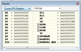
This window gives an up-to-date display of the contents of the processor registers and special function registers, and allows you to edit the content of some of the registers.
